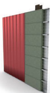
Pose ① Bardage vertical
